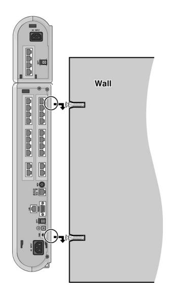
Figure 4.3.2 Wall mounting of KSU with an expansion module
